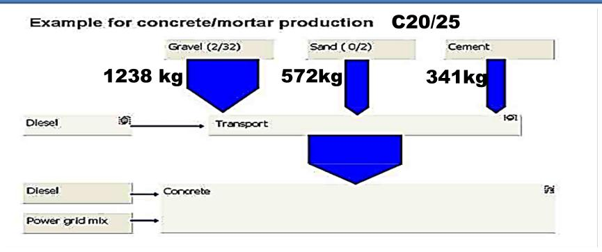
We introduced in LCA software as data elements 572kg of sand and 1238 kg of aggregates (common Gravel). Also according to the Concrete formulation C20/25 341,00kg of Portland cement.
